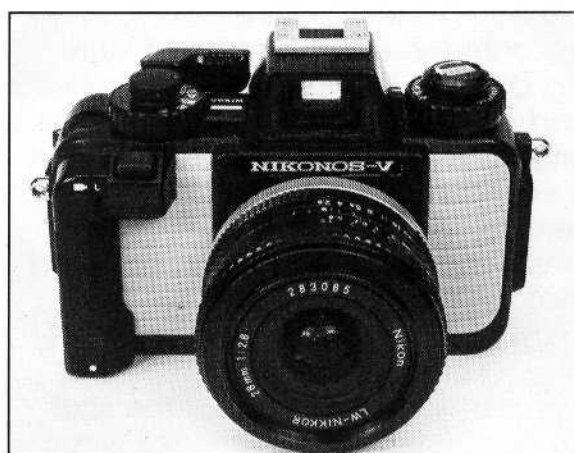
3. New 28mm land lens for Nikonos-V can withstand the elements; instruction manual for lens says to rinse lens quickly in running water without removing it from camera body to clean.
