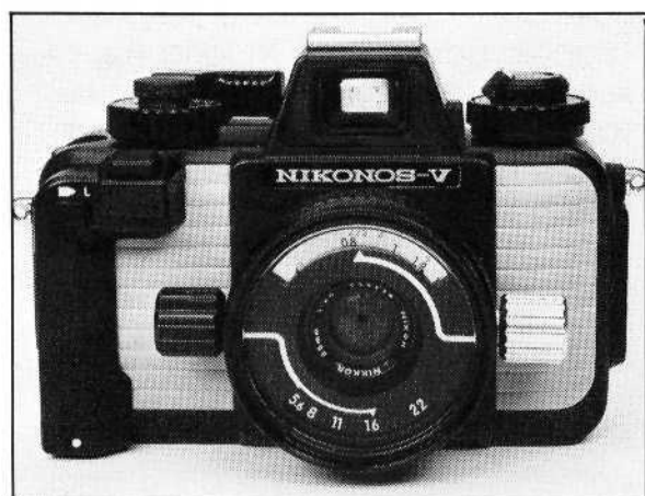
2. Standard 35mm lens can be used underwater or on land. Large silver knob is for focusing; large black knob sets the lens apertures.
